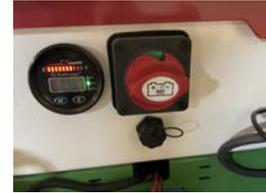
BURRO should turn on after about 5-10 seconds. BURRO's main menu should load up on the touch screen automatically. To turn BURRO OFF, just turn the same red power switch *counter-clockwise* so that it's now in the vertical position (the battery icon will be on its side) as shown above in the right image.
