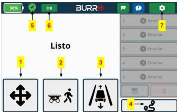
**1. Manual Control:** Opens the screen shown here. HOLD the arrow on the screen to move BURRO in that direction.
